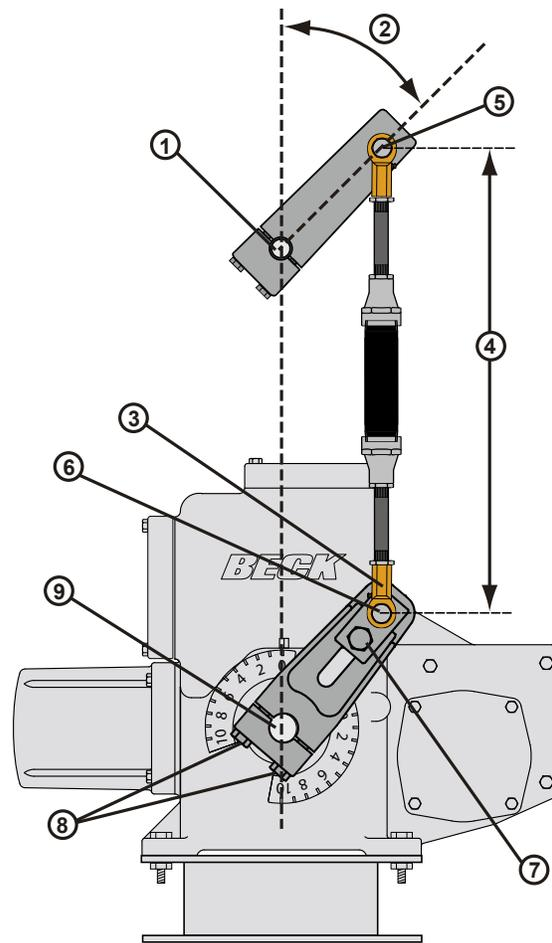
To adjust the linkage length, it is preferable to use the stud couplings. The couplings have right-hand and left-hand threads, so it is not necessary to disconnect the ends to make a length adjustment. Be careful not to expose more than 7" (178 mm) of stud between the rod end and coupling.
