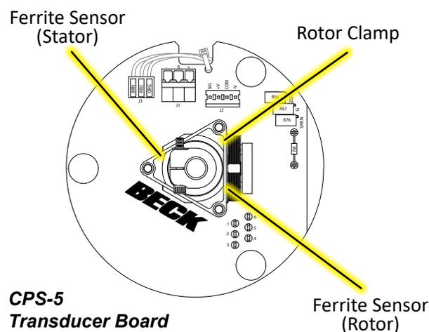
3. Record the wire colors on the terminal block of the CPS-5 (see illustration at left), then disconnect the wires. The terminals are spring-loaded. To remove a wire, press the tip of a small screwdriver into the slot at the top of the small lever. Push down to open the spring-loaded contact and release the wire.
