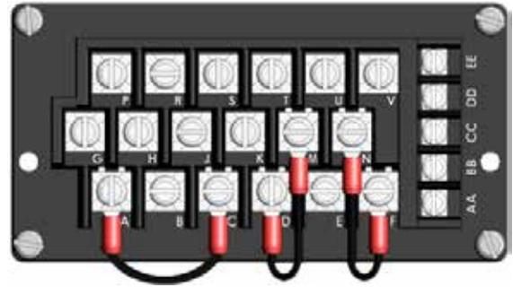
To prevent Handswitch initiated motion, remove jumper (JA) from between terminals A and C.
