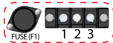
As Supplied With Optional Transformer for 208, 240, 380, 416, 480, & 575 Volts
